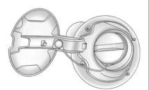
The tethered fuel cap is located behind a hinged fuel door on the driver side of the vehicle. If the vehicle has E85 fuel capability, the fuel cap will be yellow and state that E85 or gasoline can be used. See *Fuel E85 (85% Ethanol) on page 9-37.*
